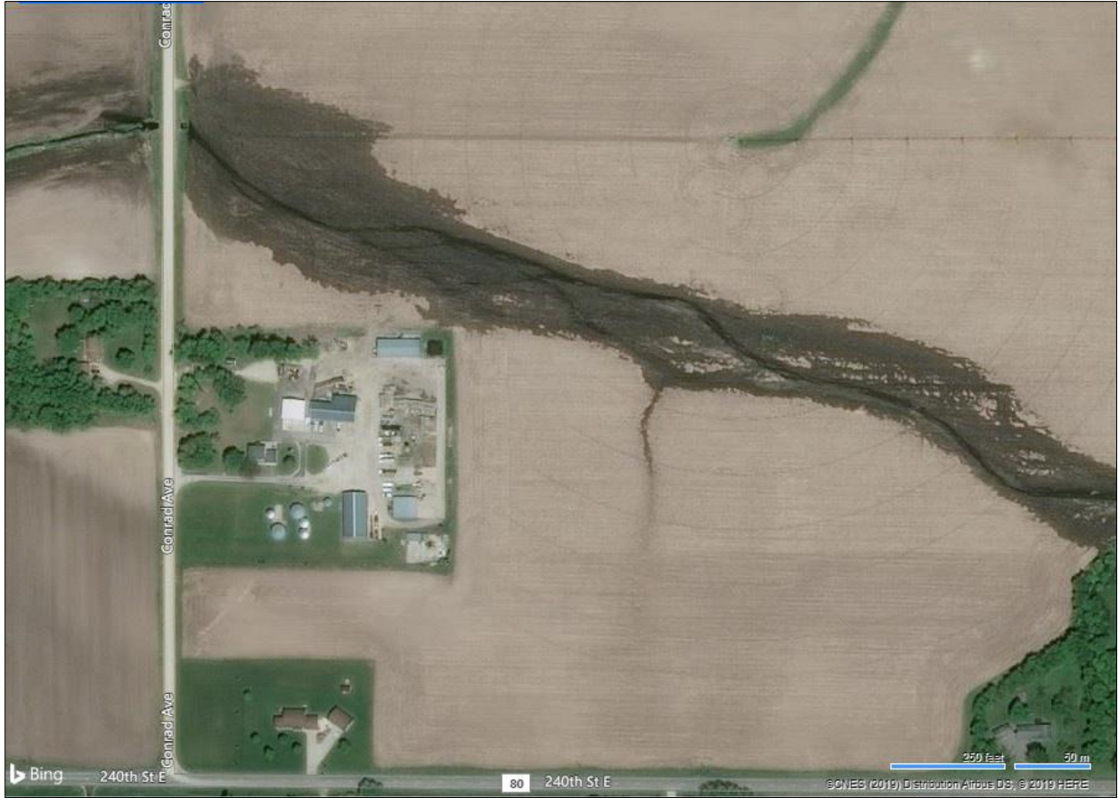
Figure 20. Example of rill erosion occurring on agricultural field.
